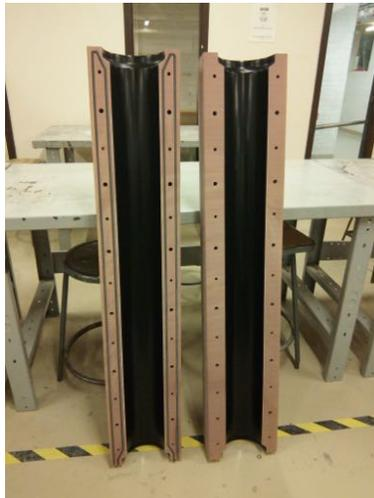
(a) Renshape molds after machining and coating.
