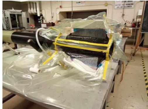
(c) Reinforcement cures under vacuum pressure.
