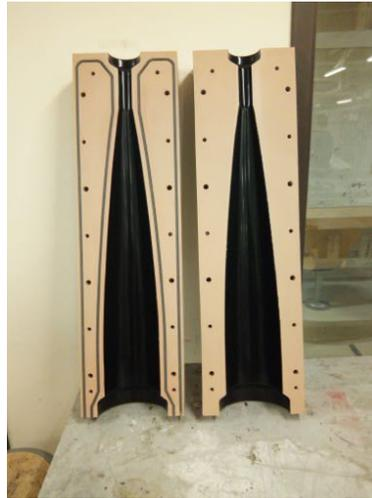
**Figure 9 Renshape nose cone molds after finishing.**
