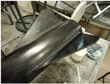
(a) Attached fin with epoxy.
