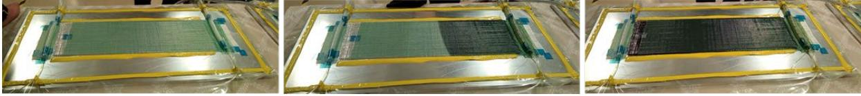
**Figure 8 Overview of the VARI process employed on a flat plate.**
