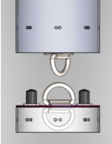
Fig. 19 Ejection Chamber with Stopper Ring and Free Plate.
