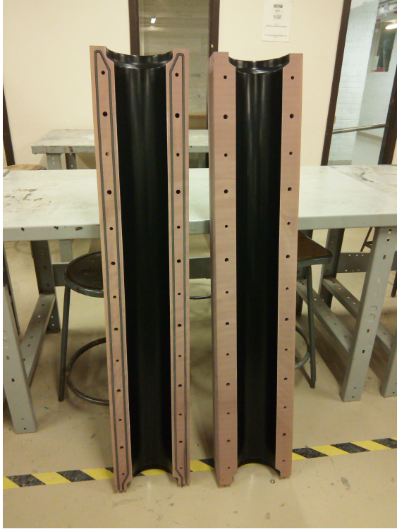
Fig. 5 Body tube mould.
