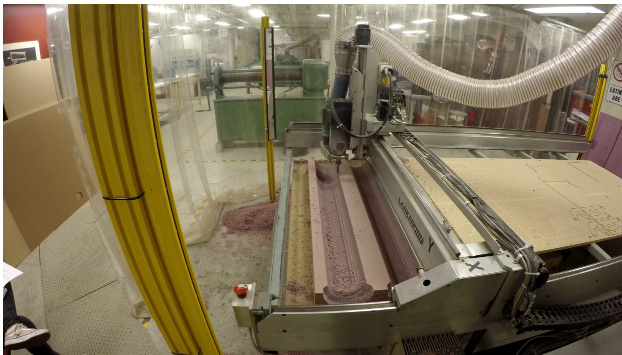
Fig. 4 Mould machining on the CNC router.
