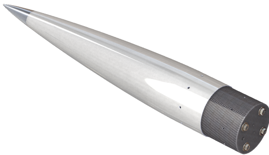
(a) von Kármán GFRP nose cone with CFRP coupler.
