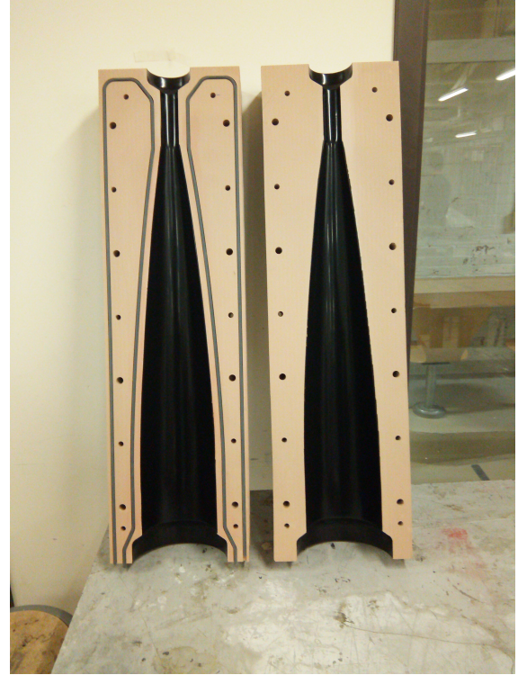
Fig. 6 Nose cone mould.
