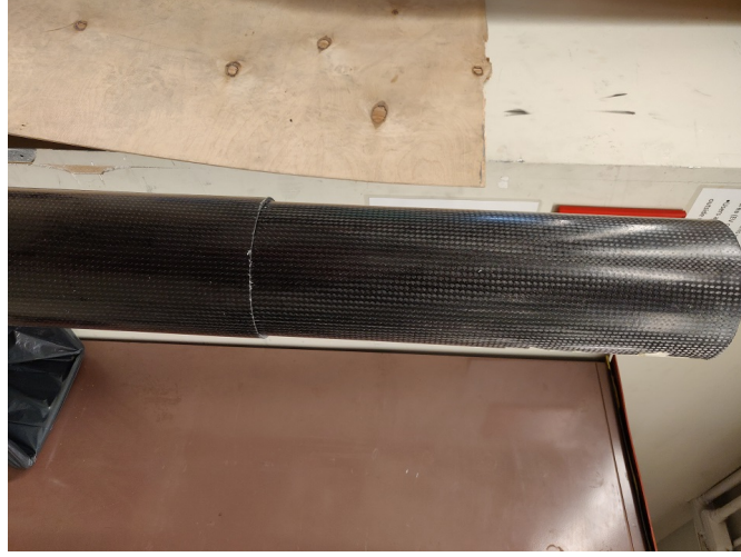
Fig. 8 CFRP body tube and coupler mating.
