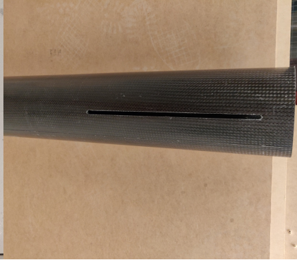
Fig. 13 Fin slits in the body tube machined using MDF jig.
